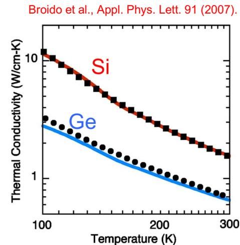
If cubic anharmonicity dominates, for  $T > T_{\text{Debye}}$  the conductivity  $k$  decreases as  $1/T$  (as experimentally observed in many low-defect “simple” crystals)
