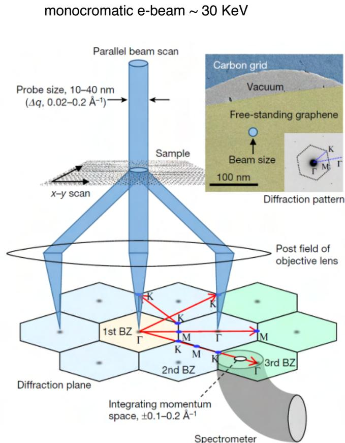
from suspended **monolayer** to ~ 20 layers (to avoid multiple scattering)
