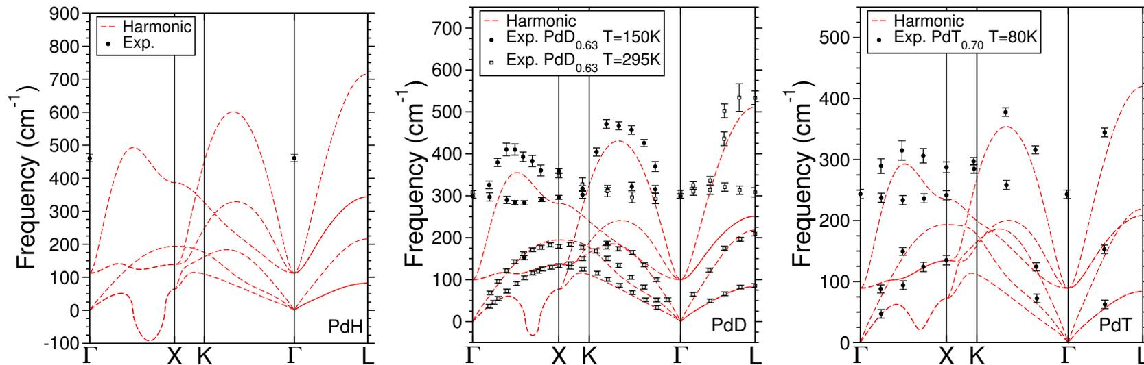
• Harmonic frequency imaginary in PdH/ and PdD and up to  $\sim 5$  times smaller than in experiment
